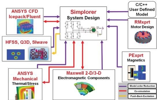
A systematic, integrated simulation approach for motor and drives systems, ANSYS Simplorer® is a multi-domain system simulation program used for designing high-performance systems that include electrical, thermal, electromechanical, electromagnetic, controller designs, etc. Simplorer ties all these different physical analyses together to ultimately optimize the whole electric powertrain as one coherent system. This figure shows the resulting design flow.
