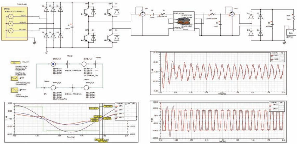
Wireless power supply system modeled in ANSYS Simplorer
