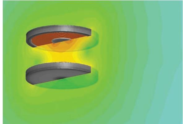
Coil antenna model (top) and magnetic field simulation using ANSYS Maxwell (bottom)
