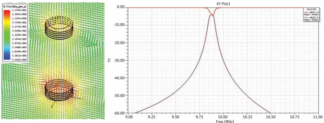
Coil antenna model (left) and results (right) using ANSYS HFSS
