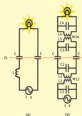
Electric power is transmitted by a series resonant system (top). The circuit for the serial system is on the left and for the parallel system is on the right (bottom).
