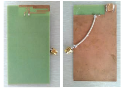
▲ Front (left) and back (right) views of the manufactured internal planar printed antenna
